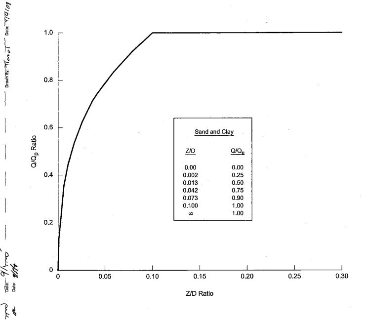
TYPICAL PILE TIP LOAD TRANSFER (Q-z) CURVES
