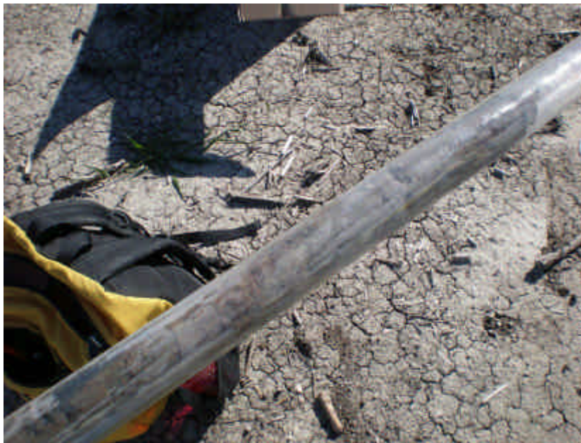
6. PA36-5, 3'-6'ft: Dark Grayish Brown Lean Clay with Sand, W% 57.5
